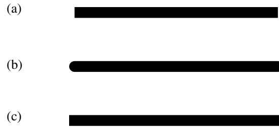
Figure 9.2: Cap styles: (a) butt, (b) round, (c) square. Note that the round and square caps protude from the start and end vertices.
